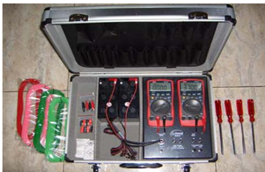
Gambar 1. Resistivitymeter tipe G-Sound (GL-4100) ( Geoelectrical Imaging , 2004).
