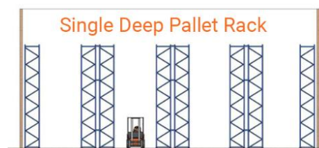
Gambar. 3 Single-Deep Pallet Rack
